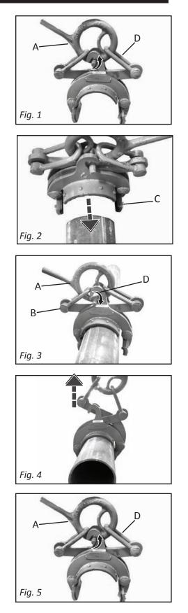
**1**. Insert lifting ring (*A*) into holding ears. (*D*, Fig. 1)
